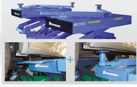
Combination of plate and swing arm makes this lift applicable to a wide range of vehicles.
